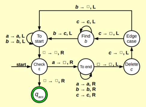
This machine works by crossing off an a from the front of the string, then going to the back of the string and deleting a c. If there are no c's left, it then tries to cross off a b. Otherwise, it deletes a second c, finds the first b it can, and replaces that b with a c. This has the effect of converting  $a^nb^nc^n$  into  $a^{n-1}b^{n-1}c^{n-1}$ . Eventually, if the string becomes empty, we accept. Otherwise, at some point we run into a mismatched or misordered symbol and reject.
